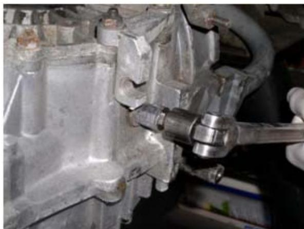
Remove the reverse light switch (22mm box end wrench), the switch activating pin (needle nose pliers), the throttle linkage bell crank (cut and remove the cotter pin), and, if the transmission has one, the small, right-angle metal bracket held by a cover nut just above the throttle bell crank. That bracket, and its strap, can be discarded; it was only used with the original clutch cable, but was determined to be unnecessary.
