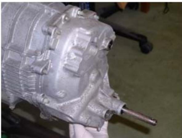
Remove the nose cover by tapping on the raised surfaces pictured with a soft mallet
