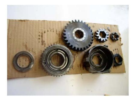
You have probably noticed numbers hand-inscribed on every gear (not on sliders). Each gear set is paired with a mate to insure long life and quiet operation; all gears must be matched by number, so if your transmission has a suspect past, now is the time to verify that nothing is mismatched.
