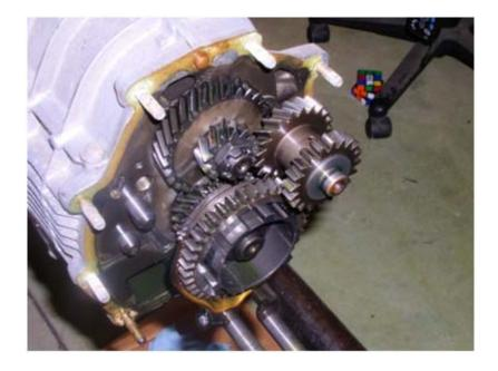
You can also see a sliding selector sleeve, the large, round gear with external and internal teeth, mounted on a shaft, for 5th and reverse, in addition to two large nuts.
