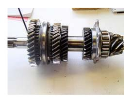
Two items worth mentioning, (1) the bearing is not on the pictured pinion shaft because at this writing I have not yet ordered it, and (2) if you have your bearing you should either install the bearing outer race into the center housing now, or put the race back in its package, label it, and put it with the pinion shaft assembly.
