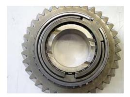
NOTE: The synchro ring for first gear is unique in that it has a groove in its two flat sides. Early rings had the groove located closer to the middle of each side; late versions have the groove as pictured above.
