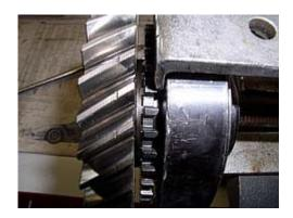
Once the dog teeth are off, clean the gear and set it on the press table. Place the new ring on the gear, wiggle it slightly, and you will feel it engage the splines on the gear. From that point, don't touch the gear or dog teeth. I carefully lower a heavy steel plate onto the dog teeth ring without letting the ring move, and then lower the press's shaft down to the plate.
