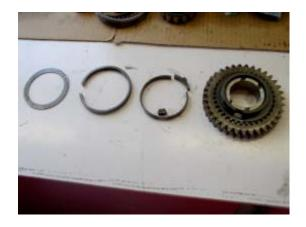
Only the retainer ring and the dimension of the installed synchro are shared with 2nd gear. Note: Beginning with the 1977 version 915/61 transmission the 1st gear dog teeth are asymmetrical in shape, while earlier 915 versions are symmetrical and use a different sliding sleeve.
