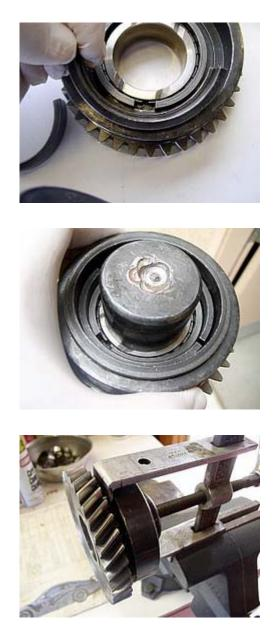
Even though a puller is designed to pull with equal force (a three jaw puller might be a better alternative than what I use, but I'm used to it), watch closely to be sure that the ring doesn't get cocked to one side.
