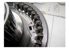
The asymmetrical teeth must face up, toward 1st gear. The asymmetrical teeth are on the same side as a machined groove on the O.D. of the slider...
