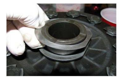
After assembly and re-installation I measured the pre-load. Remember, FAG bearings require a pre-load spec in the 30-56 lb/in range; my new reading was just over 60 lb/in, before the axle flange snapped loose and came down into the mid-50s range!
