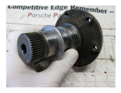
And install the flange through the side cover, into the diff...
