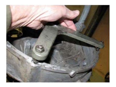
$\dots$  and install and torque the old collared nut. The torque spec is 181 lb/ft.
