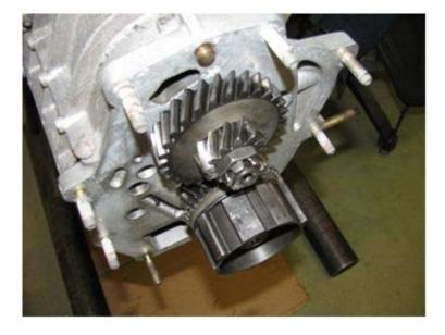
...engage the slider with 5th gear...
