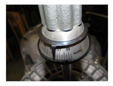
Even though pre-load was slightly out of spec, I installed the pinion shaft and measured backlash. KAZAAAM! The backlash had changed from just over .25mm all the way down to just under .10mm!
