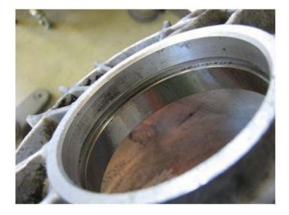
Once both bearing races are installed, insert an axle flange into the ring gear side of the diff carrier, snug the bolt, and use the flange to lower the diff into the housing. When the lower bearing is seated in its race remove the axle flange.
