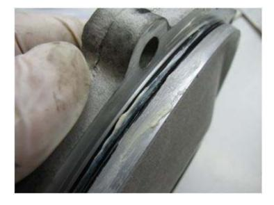
Lay the cover flat, bearing side down, and install the axle flange seal. Once again, I use grease on the seal's OD...
