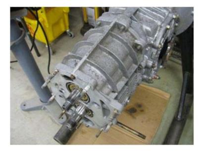
Clean and install 5th gear, along with the 5th/R slider guide...
