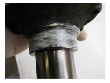
...insert the flange through the cover and into the carrier, and snug down its bolt. Torque the side cover nuts to 17 lb/ft, while turning the axle flange, and install two 8mm bolts into the axle flange. Use a screwdriver to hold the flange, and torque the axle flange bolt to 32 lb/ft.
