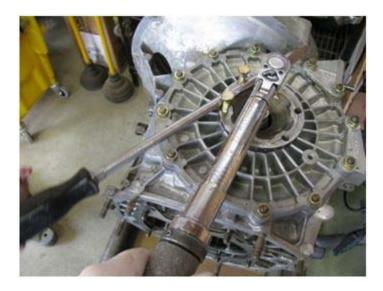
NOTE: Axle flange bolts changed during 915 production, always verify the type used on your differential, and look up the torque spec for them.
