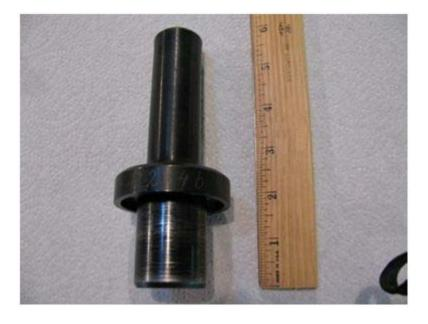
...and use the press to install the bearing. If you're doing the bearing on the side with the magnet ring, don't forget to install it after the shims and before the bearing, clean and dry, of course.
