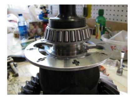
Repeat the procedure for the opposite side, but only after you; (1) install the outer race for the already installed bearing, or (2) you return the race to its box and write either, (a) speedo side, or (b) ring gear side on the box. Never use a new bearing race with; (1) an old bearing, or (2) a bearing from a different package.
