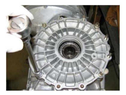
As you do this frequently turn the axle flange (with the washer in place the diff will turn with the flange), to be sure that the diff bearings aren't binding.
