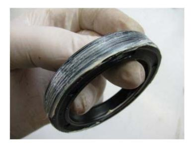
...and I use a bearing race driver and hammer to install it. Go slow with this, and when you strike the seal be aware that you can damage it. A light touch is a good thing. Also, the side cover seal is installed in a somewhat recessed position, but the opposite seal, in the housing, is installed flush with the housing.
