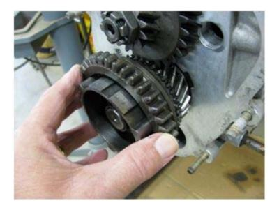
...lock the main shaft with P-tool P 37A...
