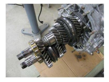
Install all ten nuts and hand-tighten them. Slide the center housing (again, we've jumped ahead a little, and I'll show you how to replace the housing's bearing races later) over the shafts, jiggle it into place, and install a couple of nuts across from each other to hold it...
