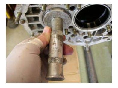
...and tap the race in. Usually no heat is required for this bearing, or the ones in the center housing, and I can't really tell you if you should use heat in a particular instance. Just use good judgment, and if a race feels too tight use a little heat, but never exceed 200 degrees F. It can't hurt, only help.
