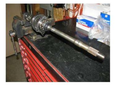
Slide your long socket onto the nut and loosen it. The torque for the collared nut is a bit more than 160 lb/ft (less on other models), so brace yourself properly. I set up the main shaft on the horizontal, block the shaft with wood, and push down on the breaker bar.
