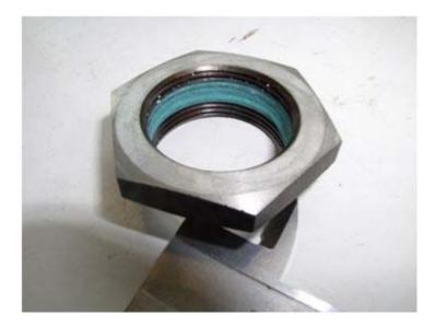
...and tighten the nut to 166 lb/ft (less on some models). Brace the shaft with a piece of wood and use a suitable punch to lock the collar into the recess machined into the shaft.
