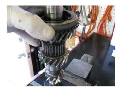
Clean and inspect the slider guide (spider) for 3<sup>rd</sup>/4<sup>th</sup> gear and install it onto the shaft. If your transmission had a big synchro failure, a broken tooth on the spider is possible. If damage (chipping, broken corners, etc.) exists the spider must be replaced. Clean and install your new shift slider; it will probably be coated with an anti-rust product, so soak it in a shallow pan of lacquer thinner in order to clean it.
