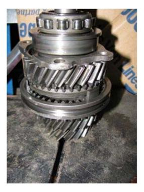
...and push the shaft down through the gear stack.
