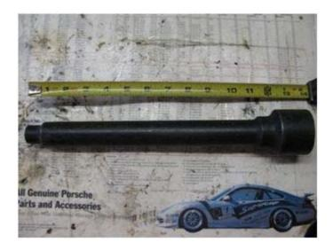
A small version of the dog tooth ring removal tool that we used on  $1^{st}$  gear is often necessary, but not nearly as frequent as the  $1^{st}$  and  $2^{nd}$  gear tool is.
