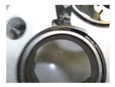
...by rotating it with a pry tool in the gap of the ring until a small screwdriver or similar can be inserted under it at the opening in the housing. Lift it carefully until it's clear of the race opening, and then gradually work it loose from its groove. Set the ring aside, turn the housing over and support it on a couple pieces of wood. Use your wheel bearing pucks, or similar, and drive the bearing race out of the housing.
