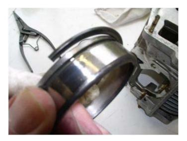
...it can be "walked" off the old race, and installed onto the new race the same way. Apply a little heat to the housing, if necessary, and tap the new race into place (note how the depth ring gap is away from the housing opening)...
