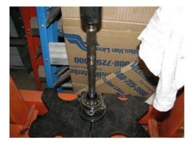
When the components are loose (like the pinion shaft, be sure to hold the main shaft firmly so it can't fall to the floor), lift the shaft with its parts from the press and re-insert it into your holder. Get out your piece of cardboard, and remove a piece at a time and place them down side down in order of removal.
