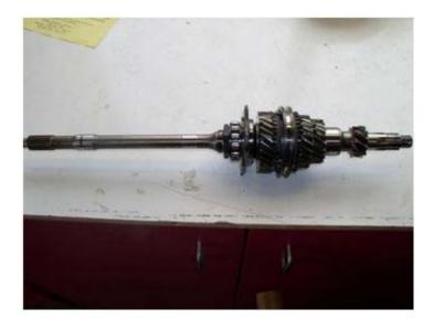
We now have a completed pinion shaft, a completed differential, and a completed main shaft. I do believe it's time to assemble the transmission, but first I'd like to show you how an inexpensive wheel bearing installation kit can help with transmission work. The last bearing that we installed on the main shaft came with an outer bearing race, and that must be tapped into place, so we'll use a puck from the kit along with a driver and hammer...
