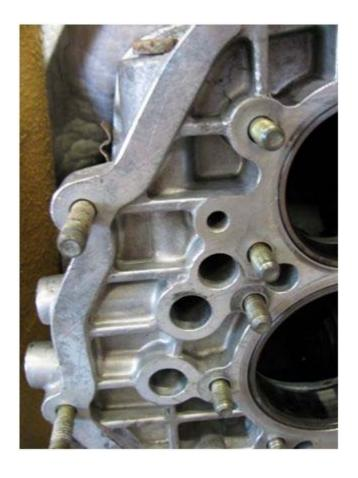
Remove the external plug (use a flat-bladed screwdriver to gently lift it, side to side, and it'll pop right out), and look down into the hole. You can see that the detent, a small piece of metal with rounded ends, drops straight down and comes to rest between the holes for the shift fork rods. Depending which gear is
