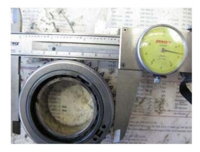
Don't forget to turn the retainer so the opening is away from the opening on the dog tooth ring, and the synchro ring. 3<sup>rd</sup> thru 5<sup>th</sup> gears use the same synchro ring, blocks and bands, and the installed spec (76.3 +/- 0.18mm) is also the same for the three synchros.
