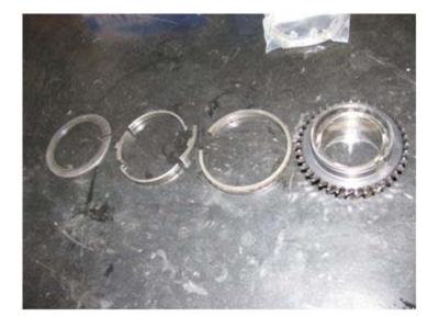
There are quantity two brake bands per gear, and the two blocks are normally called the "Energizer" block (left side in the pictures above and below) and the "Anchor" block. The brake bands are identical, and they rarely require replacement. Clean 3<sup>rd</sup> gear and its parts; reset the blocks and bands...
