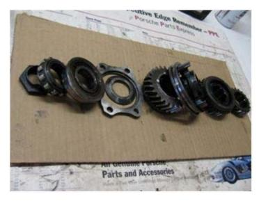
When the shaft is stripped (there is no need to remove the spacer at 2<sup>nd</sup> gear) clean it and set it back in the vise pointing up.
