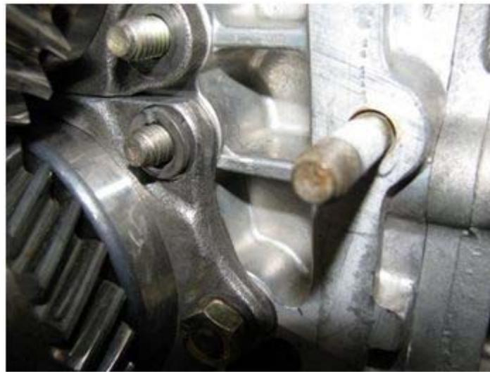
Now we're going to do something that you won't find in the books. Install your P 260A tool onto the main and pinion shafts. I discovered many years ago that by using the P 260A during clamping plate tightening, the pinion and main shafts turn smoother and easier than if they're tightened without the holder in place.
