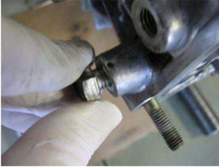
Don't worry; the above picture shows that the plug must be pushed firmly in order to compress the detent spring, and then you have to carefully align the plug with the threads to start it into the opening.
