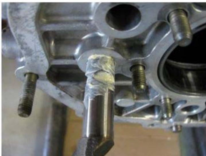
Locate a side-load detent...
