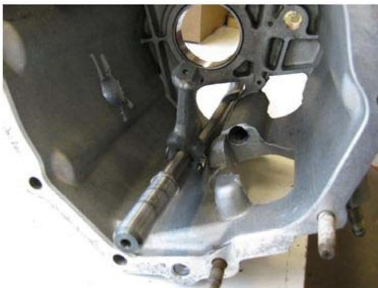
Do the same with the nose cover. Do not use any seals, gaskets or sealant.
