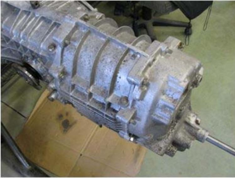
Turn over the transmission, engage the black forks with the shift rod's finger, and move the finger back and forth to make sure it fully engages both forks without hitting anywhere.
